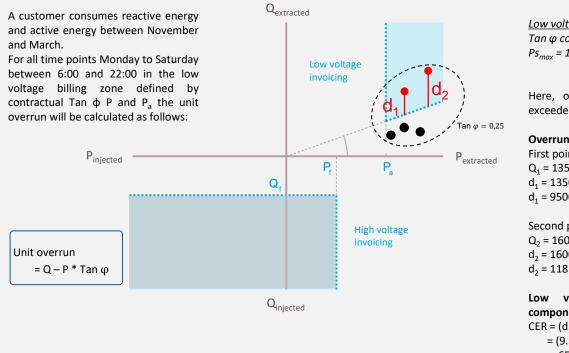
Low voltage thresholds: Tan  $\varphi$  contractual = 0.25  $Ps_{max} = 15000kW; P_a = 70\% Ps_{max}$ = 10500 kW
