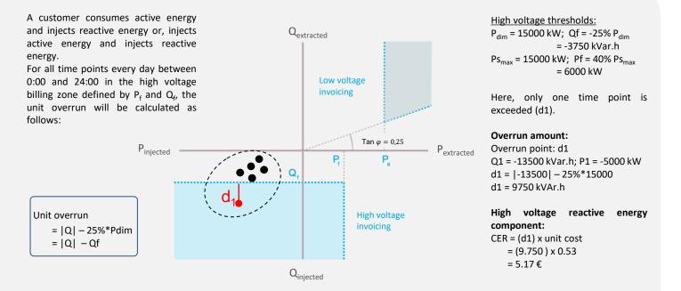
Example based on 1 August 2021 tariffs. Their value is reassessed annually. The example does not take into account the invoice capping for an overrun threshold of less than 150 MVAh/month
